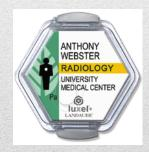
• Sensitive to x-ray, gamma, beta, and neutron radiations. The RSO also has a Luxel + OSL wrist dosimeter worn during sealed source leak testing.
