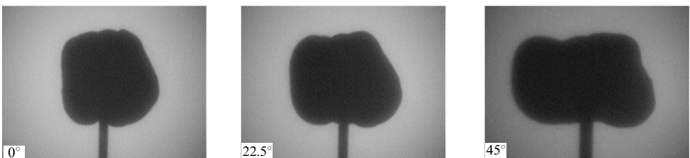
Figure 3. An illustration of the effects of changing the angle of illumination by moving the light source relative to object 1 and the projection screen.
