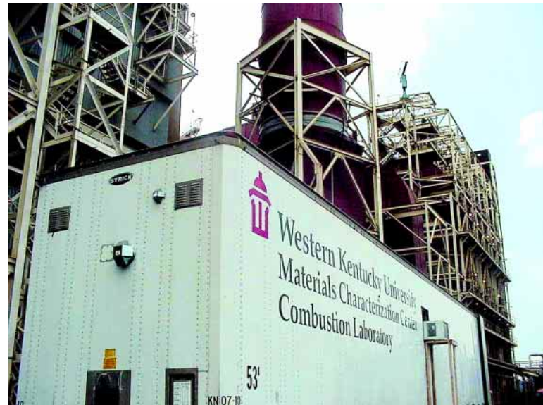
The Mobile Mercury Monitoring Laboratory, which monitors mercury emissions at regional coal-burning power plants, is a product of the Western Kentucky University Combustion Laboratory.
